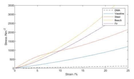
Figure 4: Stress-strain relations for a resilient interlayer tested under different friction conditions, after (Barbaresi et al., 2017).
