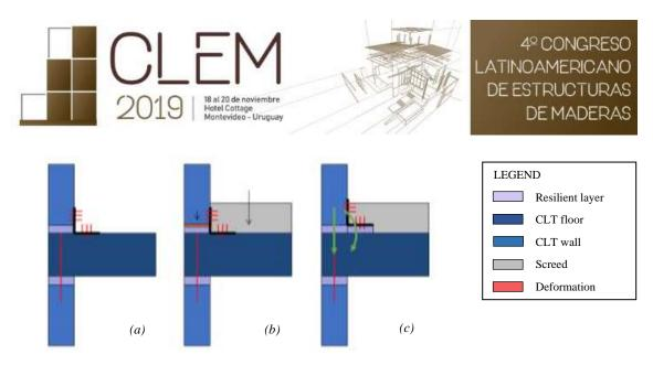
Figure 2: Schemes of CLT junction with the soundproofing profiles: (a) resilient stripes are places between timber elements; (b) the structure is loaded by permanent non-structural loads and the resilient layer is compressed; (c) the resilient layer is placed also below the metallic connectors, modifying the load transmission.
