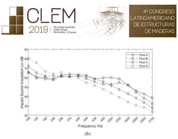
Figure 6. Normalized Impact Sound Insulation Level  $L_n(dB)$  of the construction solutions listed in Tab. 2.
